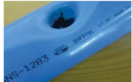
Note: Toughness of PVC-M pipes (20m High Impact test)
