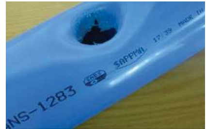
Note: Toughness of PVC-M pipes (20m High Impact test)
